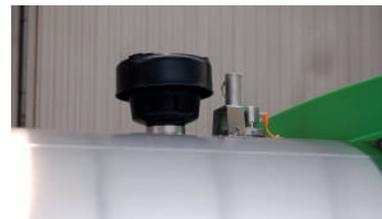
OPTICOOOL NÉCESSITE LA POSE D'UNE SONDÉ SUR LE TANK. CELLE-CI PERMET DE MESURER LE VOLUME DE LAIT PRÉSENT POUR OPTIMISER LA DURÉE DE REFROIDISSEMENT.
